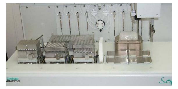
Sophas-Cat has been specially designed for Catalyst Synthesis. The synthesizer is based on an X-,Y-, Z-, pipetting station. All functions needed for synthesis, heating, cooling, mixing, vacuum filtration, powder dispensing and liquid handling are integrated into the platform. The system has 3 vortexing reaction stations, 2 with software controlled heating from ambient to  $150^{\circ}$ C, one with cooling down to  $-40^{\circ}$ C or optional  $-80^{\circ}$ C.
