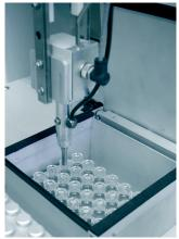
Weight reproducibility depends upon the particle size distribution within the sample. Powders with narrow particle size show precise distribution, with excellent reproducibilities. Test results with different powders have given reproducibilities of  $\pm 5\%$  for 1mg,  $\pm 3\%$  for 10mg,  $\pm 1\%$  for 50mg,and  $\pm 1\%$  for 150mg.
