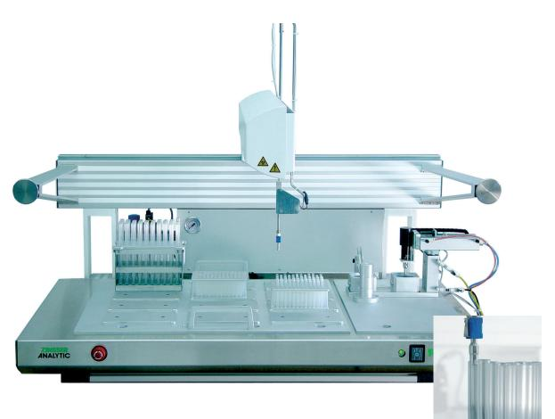
The accurate dispensing of powders is an extremely tedious and time-consuming process. REDI (Resin Dispenser), an X, Y, Z dispensing system with a powder pipet-te, helps to automate sample preparation in analytical applications, in material
